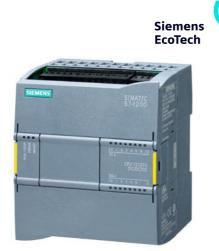
SIMATIC S7-1200F, CPU 1212 FC, compact CPU, DC/DC/DC, onboard I/O: 8 DI 24 V DC; 6 DO 24 V DC; 2 AI 0-10 V DC, power supply: DC 20.4-28.8 V DC, program/data memory 150 KB
